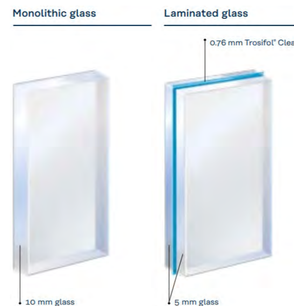
Figure 13: Example materials to replace the existing glazing on the roof canopy at Canning Town Bus Station.
