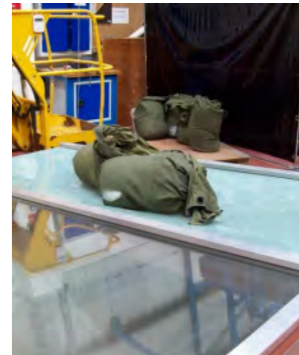
Figures 22-23: Glazing testing - photos show the 90 kg static load applied to a glass pane (left) and the underside of the sample under the static load (right).
